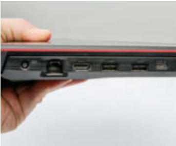
Asus-Anschlüsse links: Strom, LAN, HDMI, zweimal USB 3.1 Typ A, USB-C.
